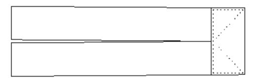
2 Side view of a folded segment. The dotted lines show where the (hidden) folds are. The teeth are at the right: the left side becomes the center of the gearwheel: the (in the drawing) upper and lower side are the sides of the gearwheel. Two segments are coupled by slitting the upper tooth of one segment in the lower tooth of the next segment. All folds of these two teeth should coincide. Closing the gearwheel (the last overlap) is the most difficult action!
